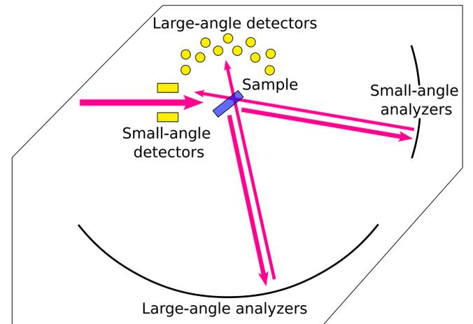
Geometry of the neutron backscattering spectrometer SPHERES at MLZ.
