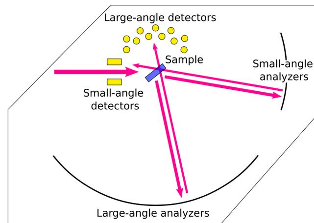
Geometry of the neutron backscattering spectrometer SPHERES at MLZ.
