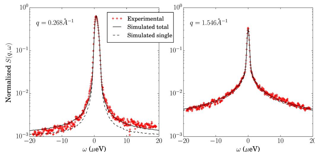
Experimental and simulated spectra at 225 K showing the difference between total and single neutron scattering for detectors at two different scattering vector lengths  $q$ .
